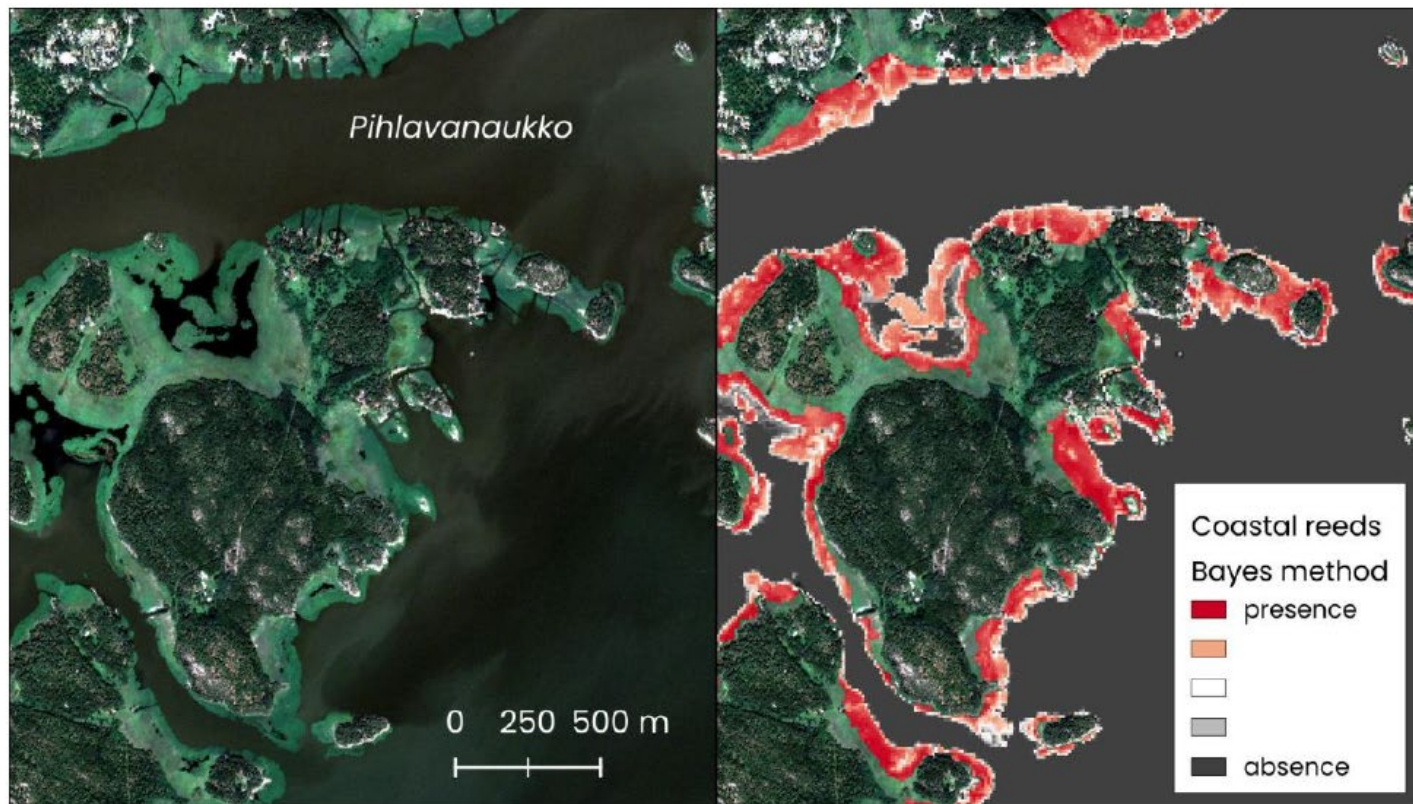
Figure 2: Left: true-colour Pléiades-1B image from the Baltic Sea coast in the municipality of Vehmaa, Southwestern Finland, in 2 July 2024. Contains modified Copernicus Contributing Mission data from the IMAGE2024 collection. Right: Same scene, overlaid with the log-likelihood of Sentinel-2 mapped pixels representing coastal reeds. The decision threshold ( \ell = 0 ) is indicated in white colour, and reddening colours have increasing likelihoods of representing coastal reeds ( \ell > 0 ). Contains modified Copernicus Sentinel-2 data, Syke (2025). Note that the method does not account for the landward side of the shoreline.
