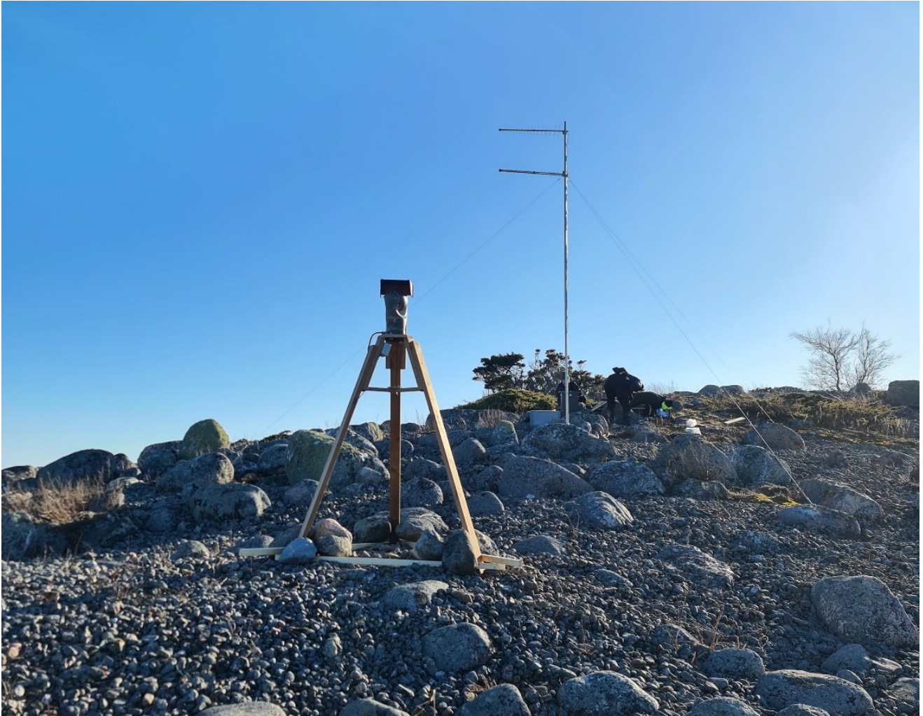
Figure 11. The live camera assembly consists of remotely rotatable and zoomable camera, power supply and data transfer system. Due to zoom and good image quality the camera can be installed far away from the shoreline without risk of degradation by the waves or water level changes.
