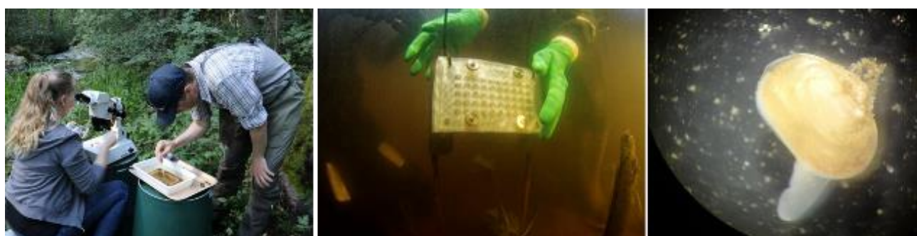
Figure 2. Buddensiek plates were used for the first restocking trial of one-year-old FPM. The mesh-covered chambers allow for natural food in the stream, and individual monitoring of mussel growth and survival (one mussel in each chamber).
