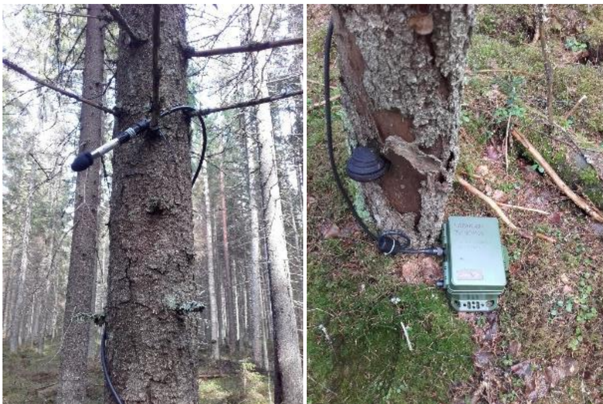
Figures 1-2. Ultrasonic microphone (left) and SongMeter 4 unit (right) were used during this action to record the ultrasound of bat calls at wetlands
